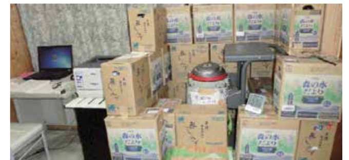
An example of trying to lower the detection limit and shorten the measurement time by using a lead and iron plate and water as an additional block. (120 kg of additional lead, 42 boxes of water totaling 250 kg)
